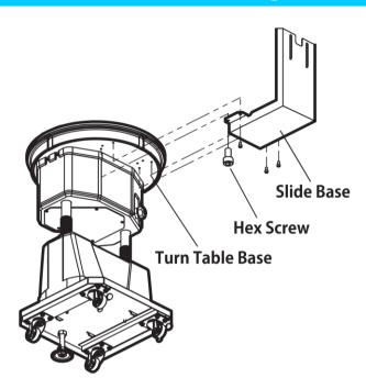
① Apply the slide base Underneath the turn table, try to align with screw holes, and using 4 screws fix the slide base to the main body.
