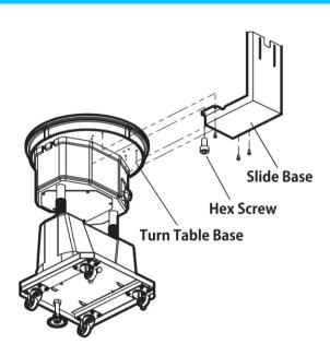
Apply the slide base Underneath the turn table, try to align with screw holes, and using 4 screws fix the slide base to the main body.
